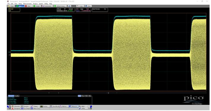
Pulsed RF carriers lie at the heart of our modern communications infrastructures, yet the shape, aberrations and timings of the final carrier pulse (at an antenna, for example) can be challenging to measure. If we choose demodulation, we are subject to the limitations of the demodulator; its bandwidth and distortions.
