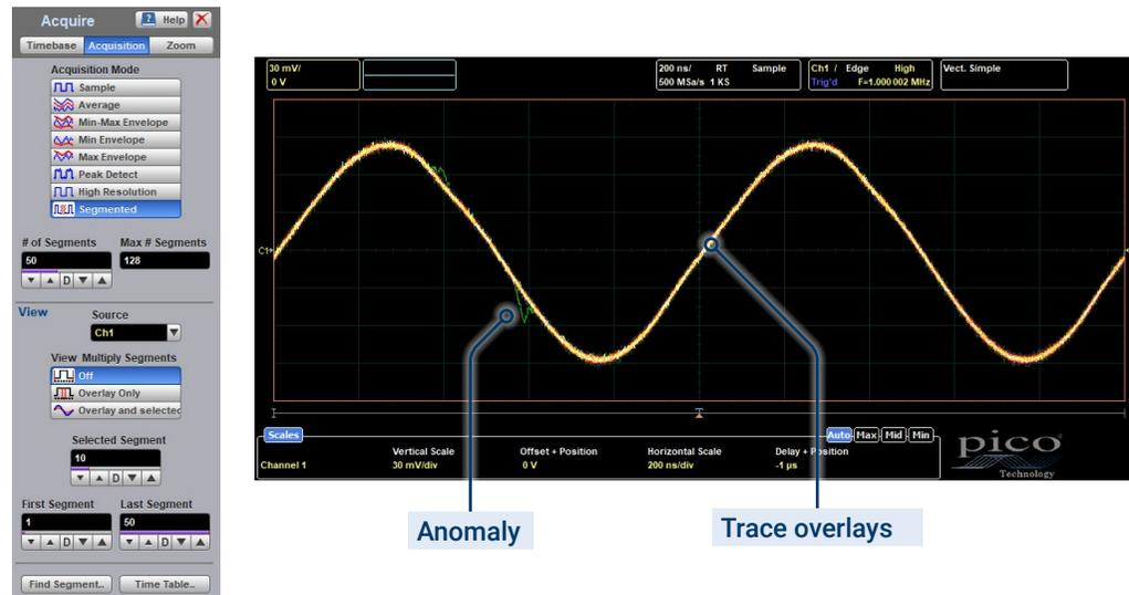
Having captured an anomalous event you can scroll through, or close gates around, an ever smaller block of overlaid traces, until the anomalous trace or traces are found. There is also a segment finder which uses a binary search method to address larger numbers of trace segments:
