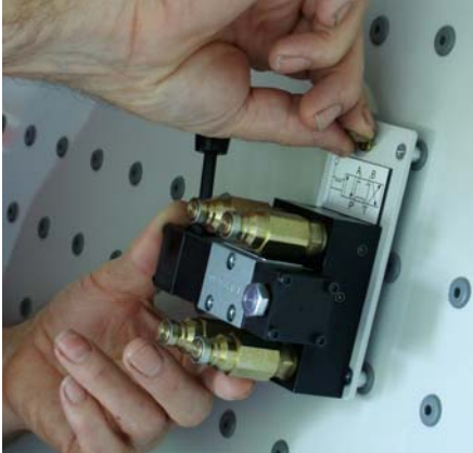
Components are easily and rapidly secured to panel using 1/4 turn fasteners
