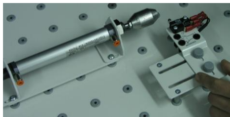
Limit switches and sensors have both horizontal and vertical adjustment
