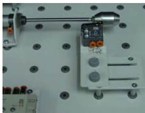
Roller valves have both horizontal and vertical adjustment
