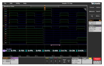
Digital channel trigger and decode
