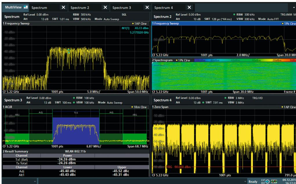
Screenshot of the R&S®FPL1000 with MultiView. The sequencer consecutively performs a spectrum measurement, an adjacent channel power measurement, a time domain measurement (zero span) and a spectrogram measurement. The results are displayed clearly and simultaneously. The toolbar on the left allows fast access to the most common menu functions. Different measurements can be activated with the tabs at the top.
