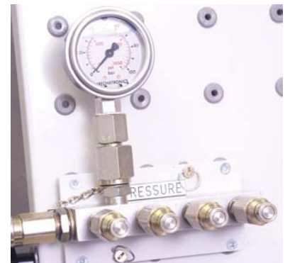
Pressure manifold showing genuine 'Flat-face' quick-release couplings
