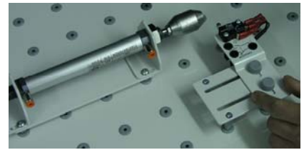
Limit switches, cylinder proximity switches and sensors have both horizontal and vertical adjustment
