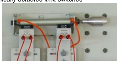
Cylinder proximity switches
