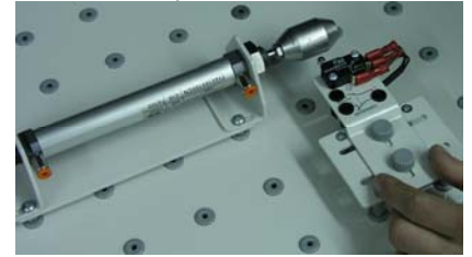
Limit switches, cylinder proximity switches and sensors have both horizontal and vertical adjustment
