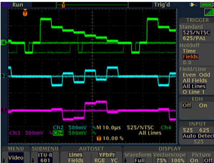
Trace and identify ITU-R BT.601 video signals with the TDS3SDI 601 Serial Digital Video Module.
